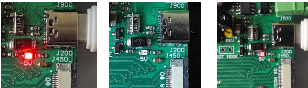
Fig. Possible LED900 states: is on (left side), is off (middle), glows dimly (right side)
