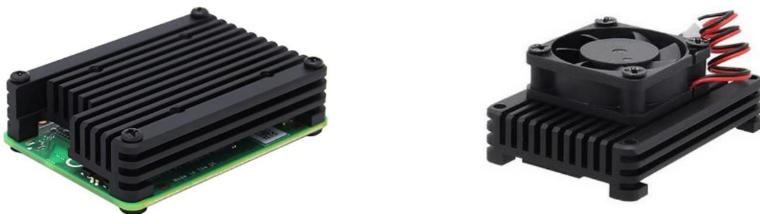
Fig. Recommended heatsink for CM4 module (left side) with optional fan (right side)
